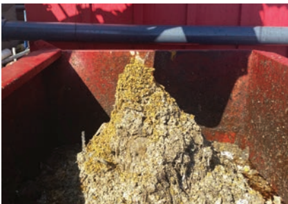
Dry, stackable debris removed from FOG loads.
