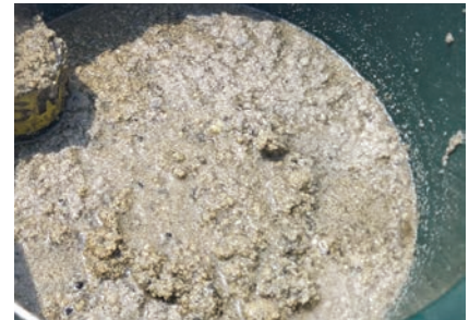
Coagulated grease with the consistency of oat meal.
